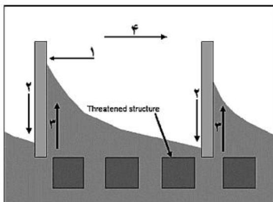
Accretion , Groin , Erosion , longshore transport direction (۱)
