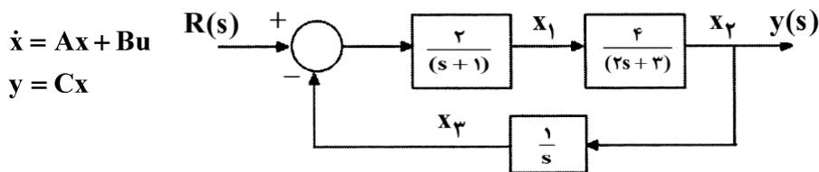
$$A = \begin{bmatrix} -1 & 0 & -2 \\ 4 & 3 & 0 \\ 0 & 1 & 0 \end{bmatrix}, B = \begin{bmatrix} 2 \\ 0 \\ 0 \end{bmatrix}, C = [0 \ 0 \ 1] \quad (1)$$
