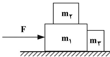
$$F_{\max} = 2\mu g(m_1 + m_2 + m_3) \text{ و } F_{\text{cont}} = 2\mu g m_2 \quad (1)$$
