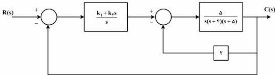
$$\dot{x} = \begin{bmatrix} 0 & 0 & 0 & -9 \\ 1 & 0 & 0 & -20 \\ 0 & 1 & 0 & -10 - \Delta k_2 \\ 0 & 0 & 1 & -\Delta k_1 \end{bmatrix} x + \begin{bmatrix} \Delta k_1 \\ \Delta k_2 \\ 0 \\ 0 \end{bmatrix} u(t), c(t) = [\Delta k_1 \quad \Delta k_2 \quad 0 \quad 0] x \quad (1)$$
