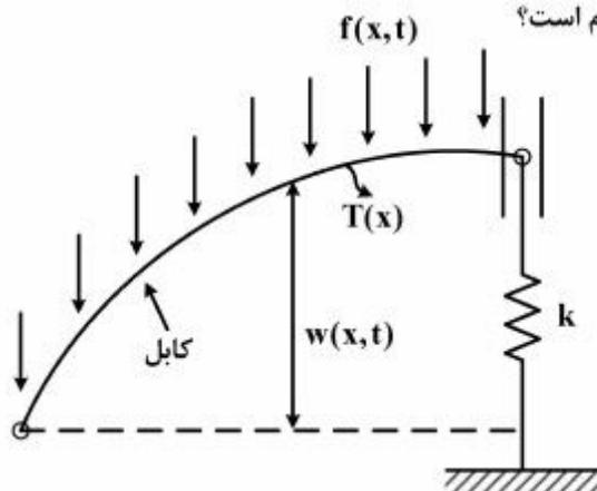
(۱)  $-\frac{\partial}{\partial x} \left[ T(x) \frac{\partial w}{\partial x} \right] + f = \rho \frac{\partial^2 w}{\partial t^2}$
