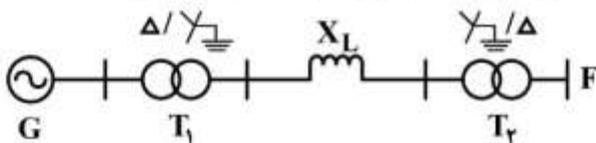
$$G \begin{cases} 50 \text{ MVA} \\ 20 \text{ kV} \\ X'' = X_r = 0.1 \text{ pu} \\ X_o = 0.5 \text{ pu} \end{cases} \quad T_1, T_2 \begin{cases} 100 \text{ MVA} \\ 20 / 132 \text{ kV} \\ X_1 = X_r = X_o = 0.1 \text{ pu} \end{cases} \quad \begin{cases} X_{L1} = X_{L2} = 0.2 \text{ pu} \\ X_{L0} = 0.5 \text{ pu} \end{cases}$$
