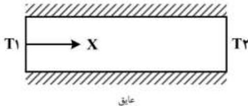
$$\frac{d^2 T}{dx^2} + \frac{1}{b} \left(\frac{dT}{dx}\right)^2 + \frac{MT}{b} = 0 \quad (1)$$
