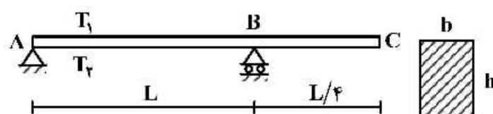
$$\frac{5}{32} \alpha L^3 (T_2 - T_1) \downarrow \quad (1)$$
